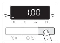
3. Using the End  $\rightarrow$  function, set the time at which the dish should be ready. In this case, 14:05.
